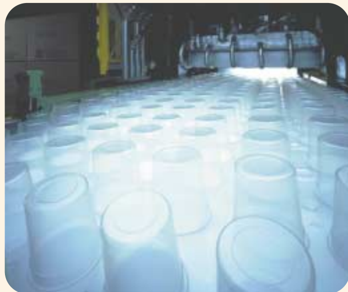
Fabri-Kal cups during manufacturing, prior to being trimmed into separate containers.
